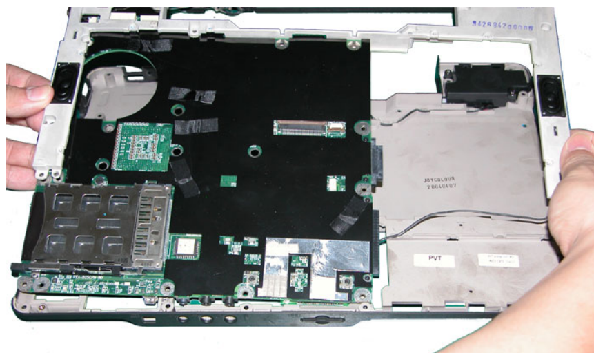
Fig. 32 Lifting up Main board
